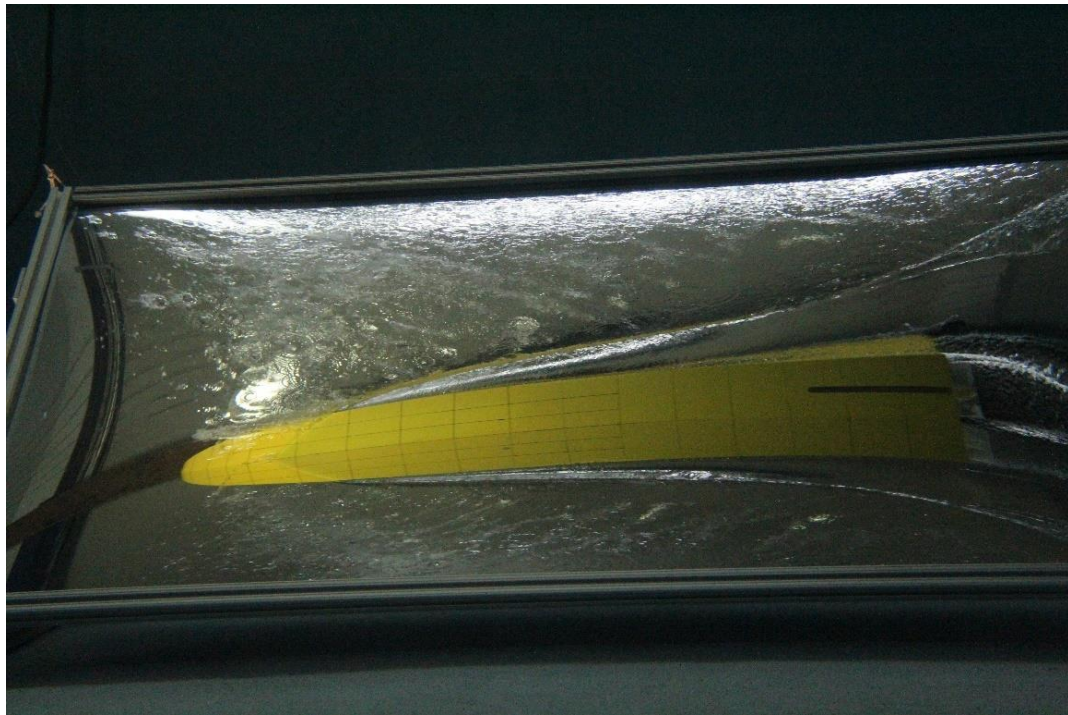
Figure 11. Underside Photo – Trim Tab C at RMB ( F_v = 2.77 )
